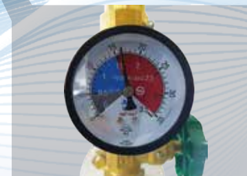
Gas Pressure Gauge
