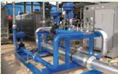
High and low pressure mixer & vaporizer
